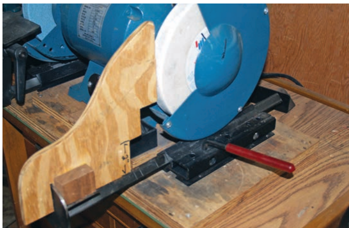
Using a simple shopmade template to set up your sharpening jig for repeatable distances saves time and tool wear.
