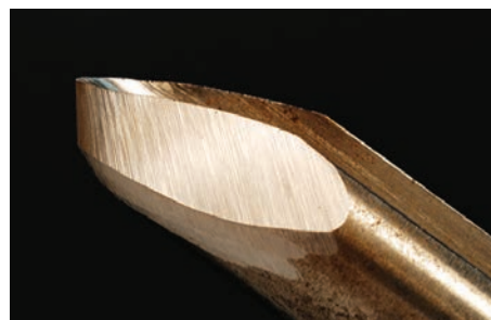
This 3/8" bowl gouge has a fingernail grind.
