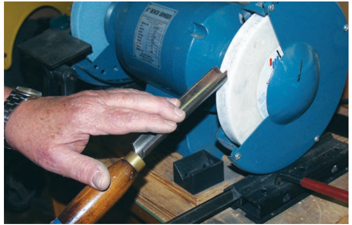
Potential danger: Using a long fixture arm and a blunt sharpening angle brings the tip of the tool too close to the wheel's equator. If the arm of the jig slips or too much pressure is exerted, it could cause the tool to jam against the wheel.
