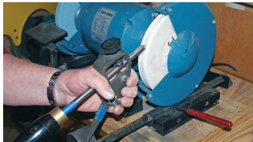
Wrong way! If the sharpening jig slips, fingers will contact the rotating wheel before the jig does.
