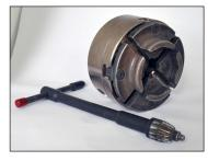
Four-jaw chucks have female threads so they can be screwed onto the threads on the spindle. When you tighten a four-jaw chuck using its key, its jaws close
