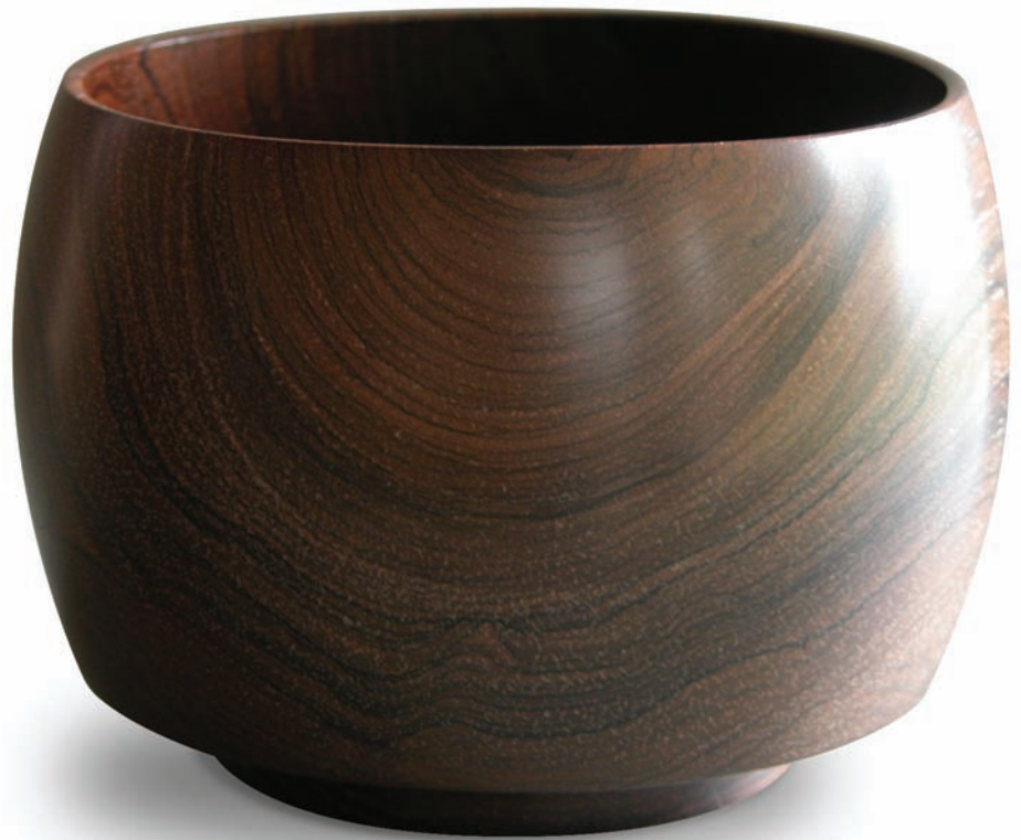
Jerry turned this 6"-diameter rosewood bowl in 1970. The wall thickness is 1/8".
